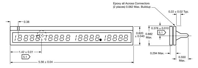
$\boxed{5.1}$  Fill tube is concentric with hole within  $\pm$  0.060 vertically and  $\pm$  0.060/- 0.030 horizontally.
