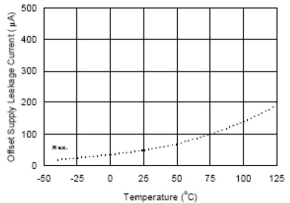
Figure 26A. Offset Supply Leakage Current vs. Temperature
