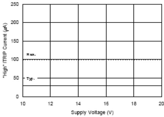
Figure 31B. "High" ITRIP Current vs. Supply Voltage
