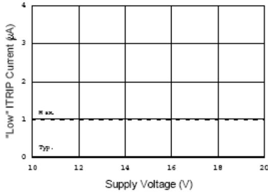
Figure 32B. "Low" ITRIP Current vs. Supply Voltage
