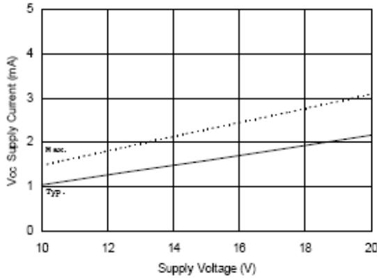
Figure 28B. V<sub>CC</sub> Supply Current vs. V<sub>CC</sub> Supply Voltage
