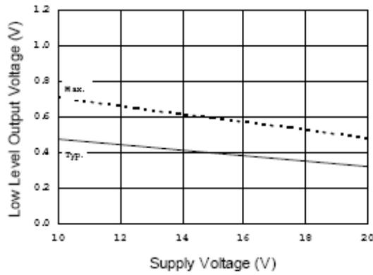
Figure 19B. Low Level Output vs. Supply Voltage
