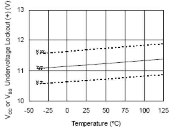
Figure 24.  $V_{CC}$  or  $V_{BS}$  Undervoltage (+) vs. Temperature (IR21363/21365/IR21366/IR21367 Only)
