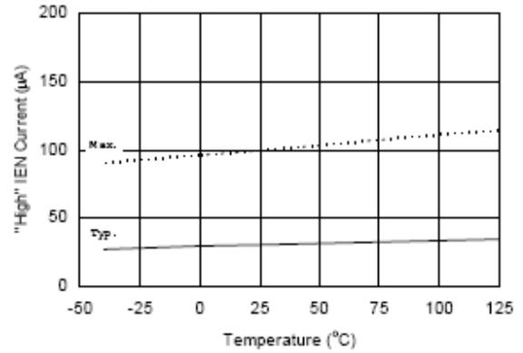
Figure 33A. "High" IEN Current vs. Temperature
