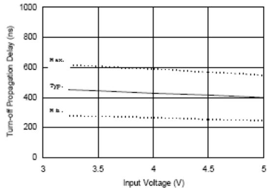
Figure 7C. Turn-off Propagation Delay vs. Input Voltage
