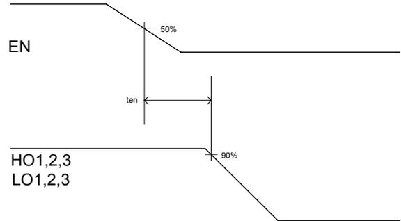
**Fig. 3. Output Enable Timing Waveform**
