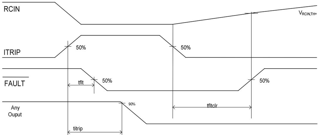
**Fig. 5. ITRIP/RCIN Timing Waveforms**
