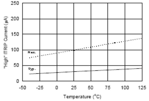
Figure 31A. "High" ITRIP Current vs. Temperature
