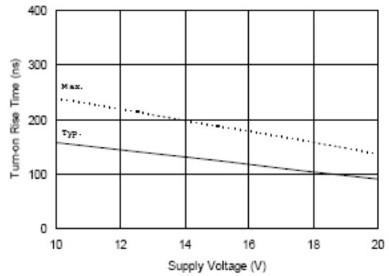
Figure 8B. Turn-on Rise Time vs. Supply Voltage
