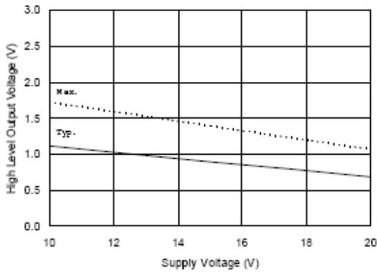
Figure 18B. High Level Output vs. Supply Voltage
