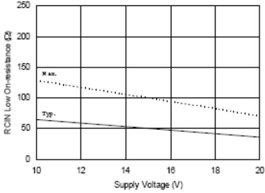
Figure 38B. RCIN Low On-resistance vs. Supply Voltage
