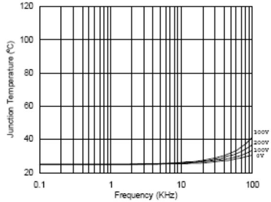
**Figure 46. IR2136/IR21362(3)(5)(6)(7)(8) (J) vs. Frequency (IRG4BC30W), Rgate=15Ω, Vcc=15V**
