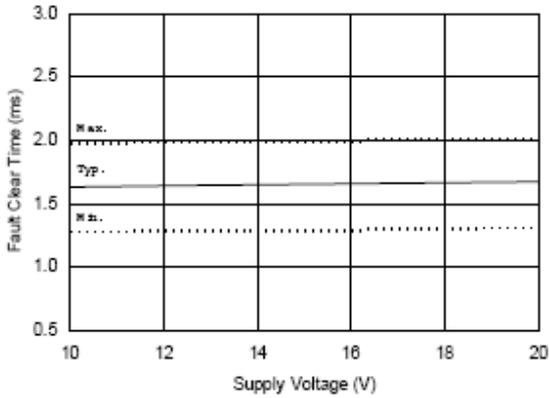
Figure 13B. FAULT Clear Time vs. Supply Voltage
