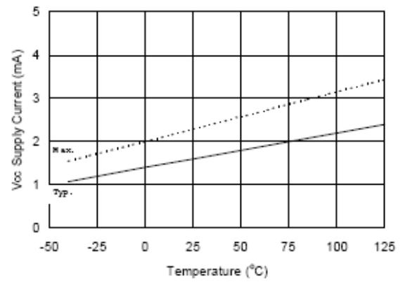
Figure 28A. V<sub>Cc</sub> Supply Current vs. Temperature
