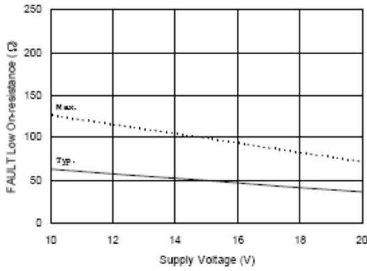
Figure 39B. FAULT Low On-resistance vs. Supply Voltage
