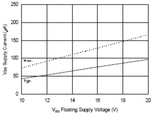
Figure 27B. V<sub>Bs</sub> Supply Current vs. V<sub>Bs</sub> Floating Supply Voltage
