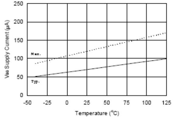
Figure 27A. V<sub>Bs</sub> Supply Current vs. Temperature
