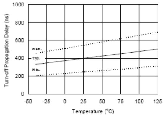
**Figure 7A. Turn-off Propagation Delay vs. Temperature**
