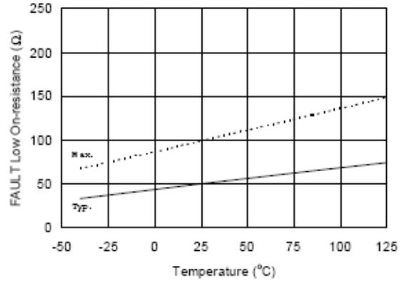
Figure 39A. FAULT Low On-resistance vs. Temperature
