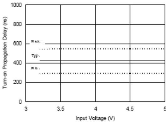
**Figure 6C. Turn-on Propagation Delay vs. Input Voltage**
