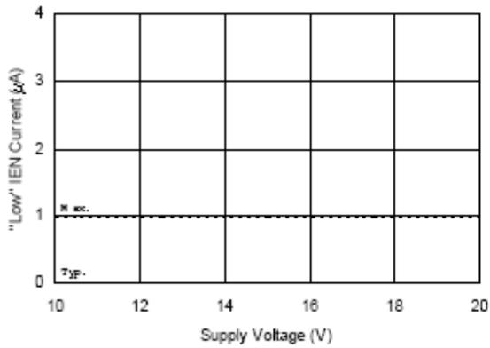
Figure 34B. "Low" IEN Current vs. Supply Voltage
