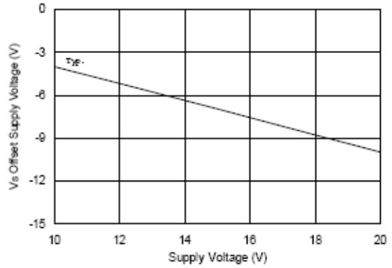
Figure 40. Maximum Vs Negative Offset vs. VBS Supply Voltage
