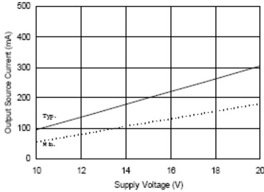
Figure 36B. Output Source Current vs. Supply Voltage
