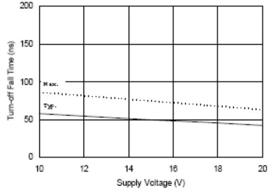
Figure 9B. Turn-off Fall Time vs. Supply Voltage
