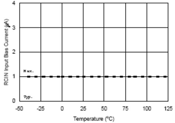
Figure 35A. RCIN Input Bias Current vs. Temperature
