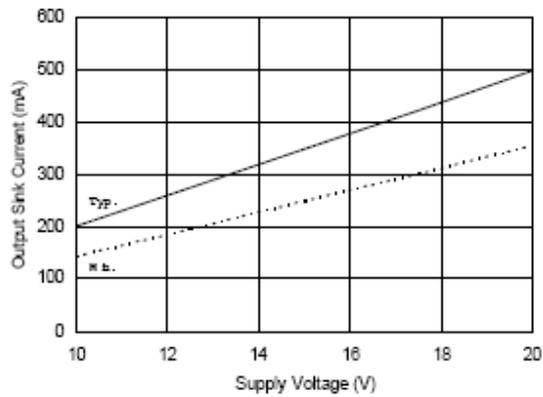
Figure 37B. Output Sink Current vs. Supply Voltage
