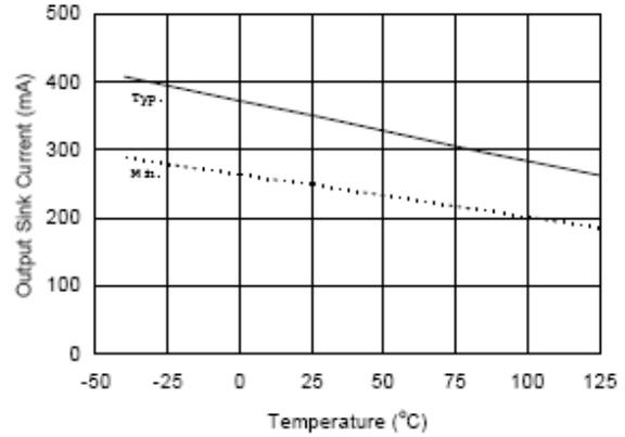
Figure 37A. Output Sink Current vs. Temperature
