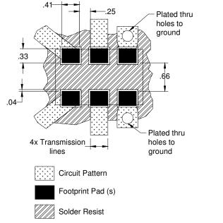
Dimensions are in Millimeters Mounting Footprint
