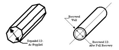
Typical applications are where tubing must fit over a large object such as in the repair or replacement of cable jacketing.
