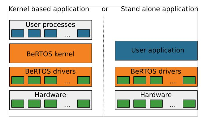
Hardware drivers are supported on many different architectures with a single API. This result is achieved using an abstraction over the physical hardware.
