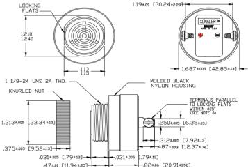
NOTE A: TERMINALS-.032 BRASS TIN PLATED, TAPPED FOR #6-32 SCREW, TWU #6-32 NICKEL PLATED BRASS SCREWS INCLUDED, WILL ACCEPT 1/4\* QUICK CONNECT. NOTE B MOUNTING- REMOVE BLACK PLASTIC NUT
