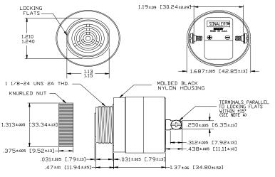
NOTE A: TERMINALS-.032 BRASS TIN PLATED, TAPPED FOR #6-32 SCREW. TVOI #6-32 NICKEL PLATED BRASS SCREWS INCLUDED. WILL ACCEPT 1/4" QUICK CONNECT. NOTE B: MOUNTING- REMOVE BLACK PLASTIC NUT AND INSERT THREADED FRONT THROUGH 1.25' HOLE PUNCHED IN PANEL, IF ORIENTATION IS NEEDED, NOTE LOCKING FLATS ON DRAWING. SCREW NUT BACK ON. DO NOT OVERTIGHTEN.
