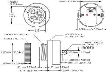
NOTE A: TERMINALS-.032 BRASS TIN PLATED, TAPPED FOR #6-32 SCREW. TWO #6-32 NICKEL PLATED BRASS SCREWS INCLUDED. WILL ACCEPT 1/4' QUICK CONNECT. NOTE B: MOUNTING- REMOVE BLACK PLASTIC NUT AND INSERT THREADED FRONT THROUGH 1.25' HOLE PUNCHED IN PANEL, IF DRIENTATION IS NEEDED, NOTE LOCKING FLATS ON DRAVING, SCREW NUT BACK ON. DO NOT OVERTIGHTEN.
