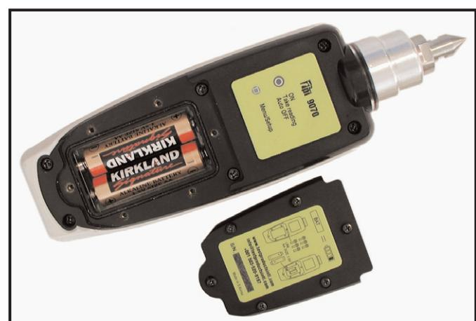
Care must be taken when the batteries are changed. Make sure the gasket is properly seated when reinstalling the battery door otherwise the IP67 rating will be compromised.
