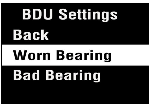
The BDU threshold values are designated as Worn Bearing (where readings turn **Amber**) and Bad Bearing (where readings turn **Red**).
