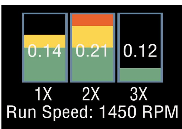
Pressing the square button brings up a display similar to that shown opposite, which shows the readings of vibration velocity (mm/s or inch/s) broken down into each of 3 bands.
