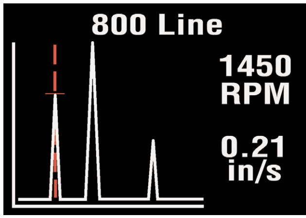
The heights of the peaks indicate the RMS vibration level in (mm/s or inch/s) at each frequency point in the spectrum.
