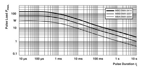
Maximum pulse load, single pulse; for permissible resistance change equivalent to 8000 h operation. **Single Pulse**
