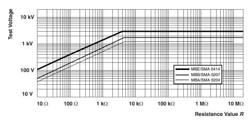
Pulse load rating in accordance with IEC 60115-1, 4.27; 10 μs/700 μs; 10 pulses at 1 minute intervals; for permissible resistance change (0.5 % R + 0.05  $\Omega$ )
