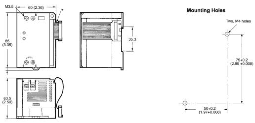
\*A flat cable with a length of 85 mm can be used.
