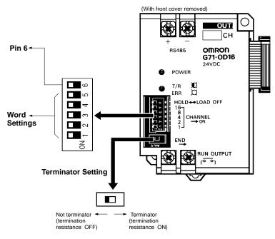
Note: The terminator setting also sets the termination resistance. Be sure to set only one terminator per Remote I/O Master Unit and be sure it is the Unit farthest from the Master. (Set to OFF at the factory). Set word numbers in backwards order from 31. (Set to 31 at the factory). See G72C-5 for system configurations and operating precautions.
