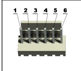
**PGED2** conducts I/O operations for the “Program Data” signal. Serial data for programming.
