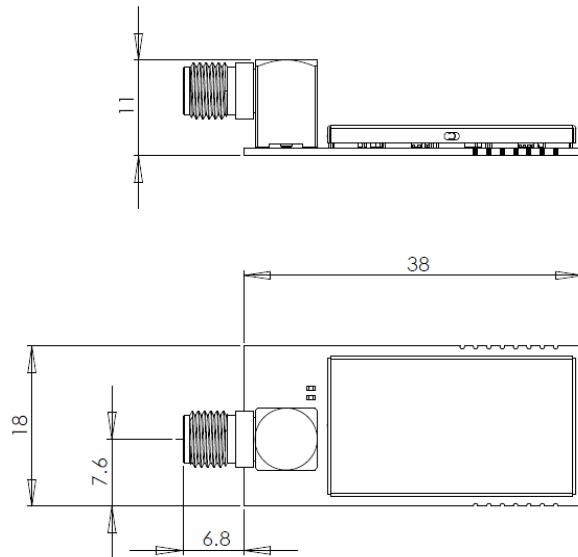
**Module with Chip Antenna dimensions (mm):**
