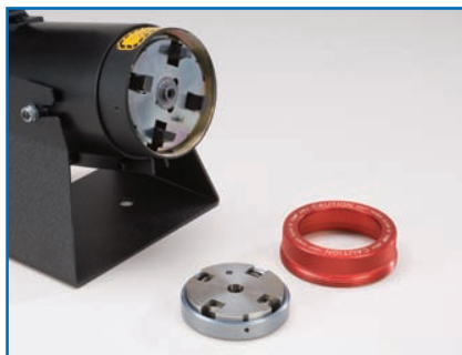
2. Pull off Indenter Die Assembly by hand.
