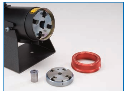
3. Pull out the Locator by hand.
