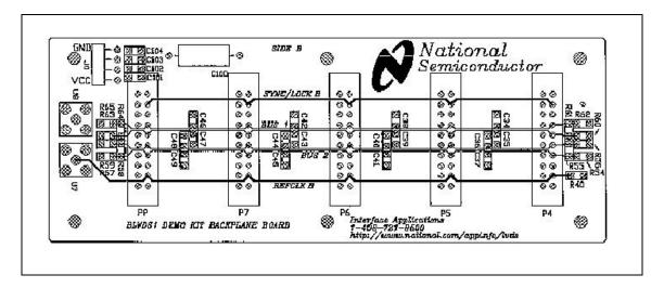
Each side of the backplane card has two differential busses, a REFCLK bus to distribute the REFCLK signal to deserializer cards, and a SYNC/LOCK bus that connects the LOCK\* output from deserializers to the SYNC1 input of the serializer.
