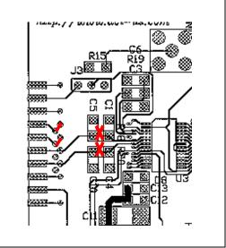
1. On the DUT card, side A, solder a jumper from the R16 pad to the inside pad of C30.
