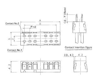
Note: The dip side may be deviated according to the cable thickness and the crimping contact bent up/down.
