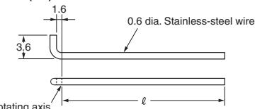
**D2MC****Low-Torque Basic Switch**D
