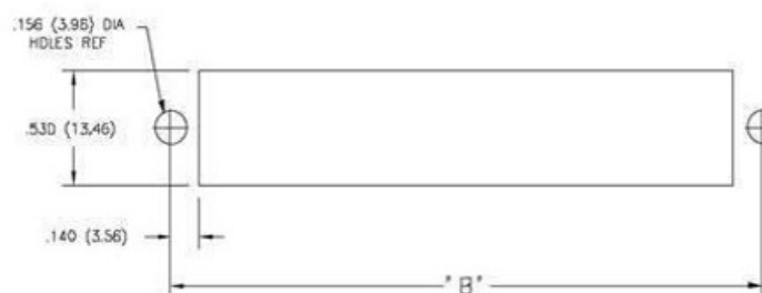
CONNECTOR MOUNTING PATTERN PANEL MOUNT OUT OUT
