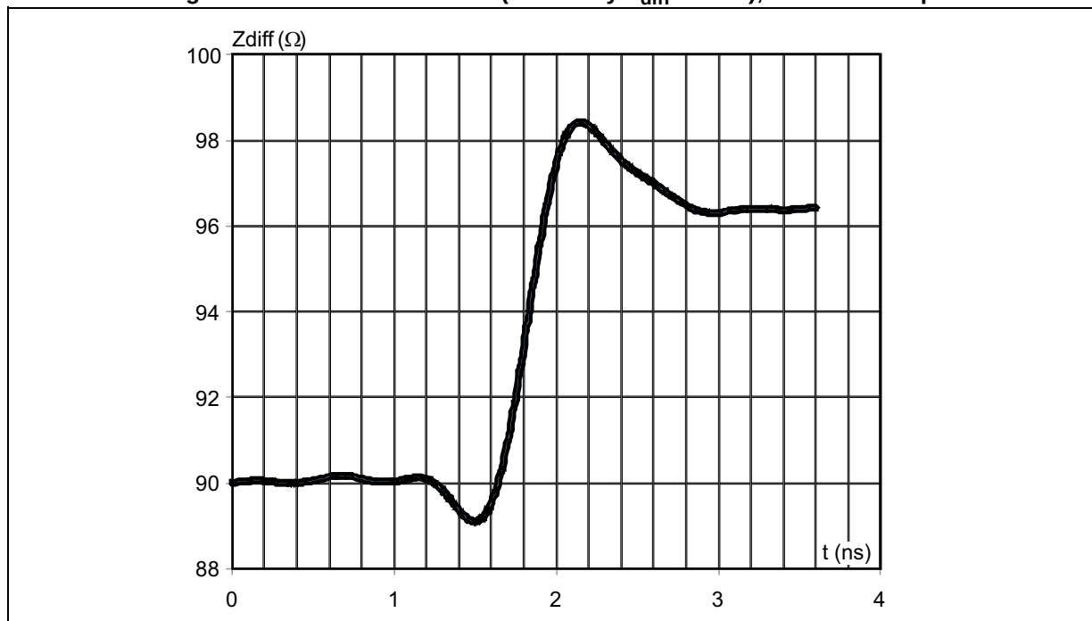
Figure 16. TDR measurement (loaded by Z_{diff} = 90 \Omega ), rise time 400 ps
