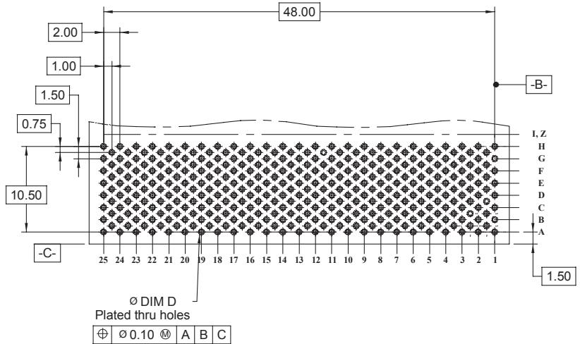
Recommended PCB hole mounting pattern for coaxial,
