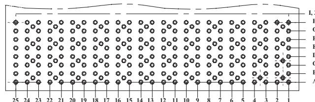
Recommended PCB hole mounting pattern for row
