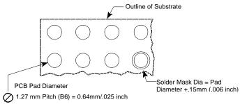
For .006" Thick Solder Paste Stencil, Aperture Opening Should be Equal to the PCB Pad Diameter.
