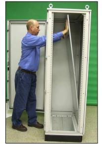
D) Continue to push the top of the panel until the collar studs protude through the panel mounting holes. Ensure the pins protrude through the bottom of the panel supprts.
