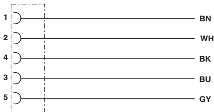
Contact assignment of the M12 socket
