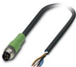
Sensor/Actuator cable, 4-position, PVC, Black RAL 9005, Plug straight M8, on Free cable end, Cable length: 5 m
