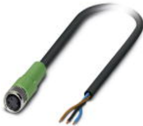
Sensor/Actuator cable, 3-position, PVC, Black RAL 9005, Free cable end, on Socket straight M8, Cable length: 10 m
