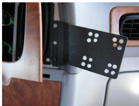
InDash fit into location with screw
