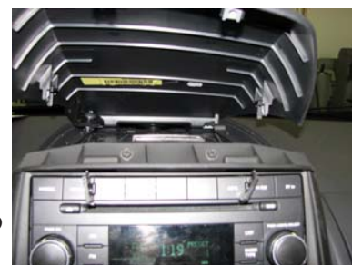
Cover Removal and screws under cover
