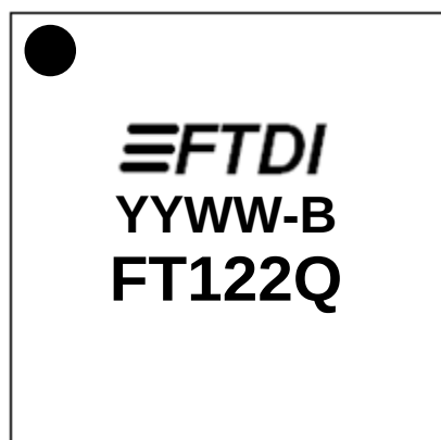
Figure 9-4 QFN-28 Package Markings
