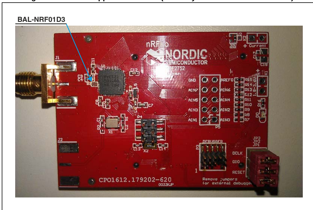
Figure 9. nRF2752 application board (courtesy of Nordic Semiconductor)
