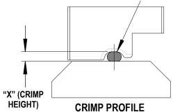
Use pin gauge or soft metal slug (solder) method to measure the "X" dimension. Verify tooling crimp height calibration by referring to the Go/No Go dimensions shown in the chart below.
