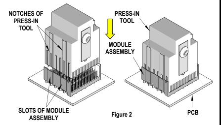
3. Using the application tool and an appropriate press, seat the header assembly until there is less than 0.10mm (.004 in) clearance between the bottom of the plastic housing and the surface of the PCB. See Figure 3.
