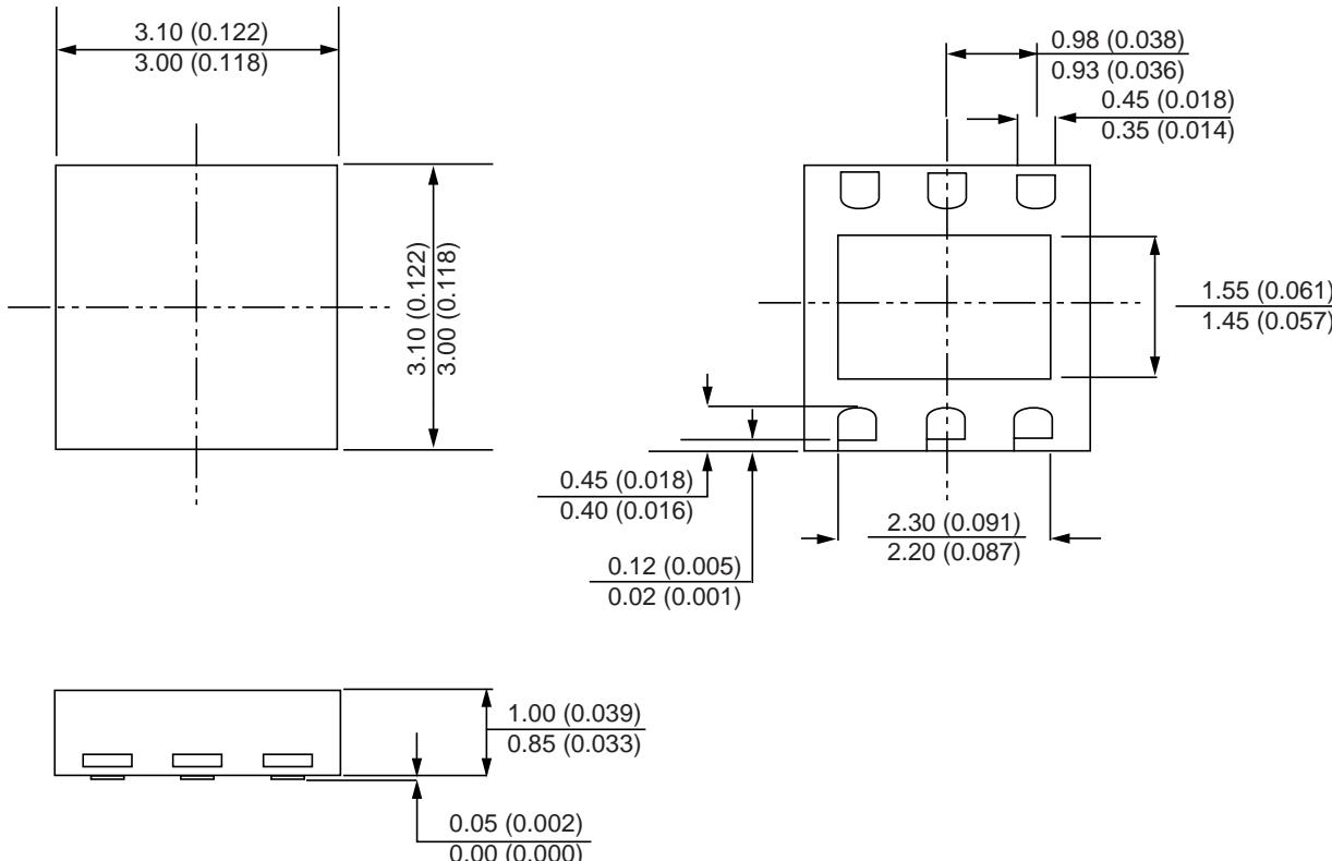
**Note:** The PLLP6 package has thermal power dissipation of 320°C/Watt in free air. Attaching the package to a circuit board improves thermal performance. Dimensions are in mm (inches).
