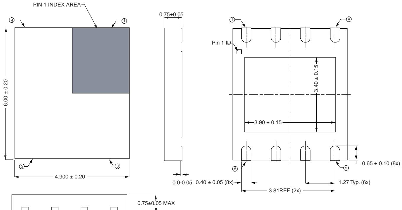
Note: Dimensions in mm. TDFN SO8 Package has thermal power dissipation of 240°C/Watt in free air. Attaching the package to a circuit board improves thermal performance.
