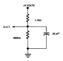
\* INCLUDING SCOPE AND JIG CAPACITANCE
