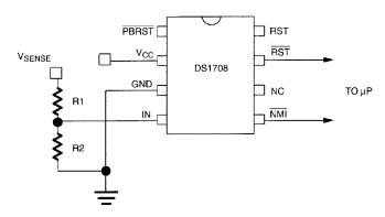
$$V_{SENSE} = \frac{R1 + R2}{R2} \times 1.25 \qquad V_{MAX} = \frac{V_{SENSE}}{V_{TP}} \times V_{CC}$$
