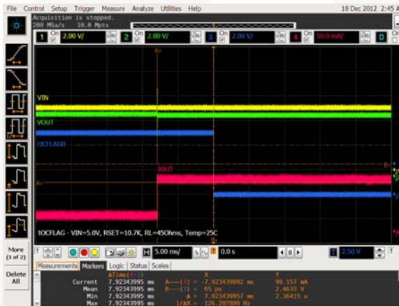
Figure 8. t_{OC\_FLAGB} Response Time (Toggle R_{LOAD} from High to Low Resistance)
