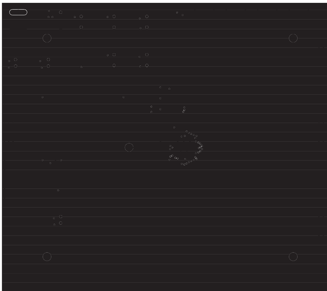
Figure 4. MAX3673 EV Kit PCB Layout—Ground Plane
