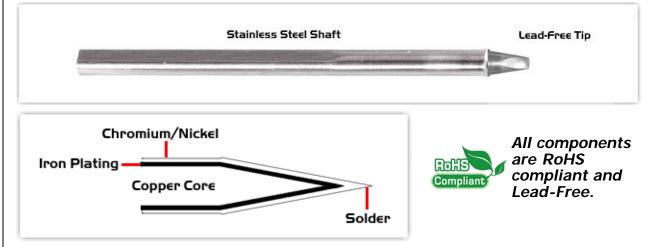
Easy Braid Co. tip cartridges will typically idle within a temperature range of +/-1.1°C. However, there is variation in idle temperature across tip geometries within an individual temperature series. Easy Braid Co. offers a wide variety of tip geometries from 0.25mm fine point tip to 5mm chisel. The length and geometry of a tip will have an influence on the tip idle temperature. To accurately measure idle temperature it will depend greatly on the measurement method,
