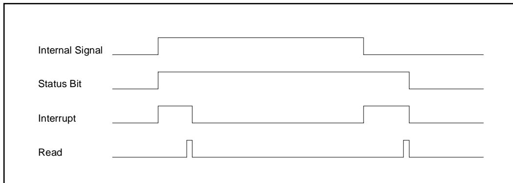
Figure 4-2. Alarm Status Bit
