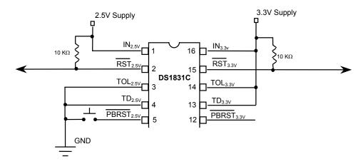
NOTE: If outputs are at different voltages the outputs can not be connected to form a wired AND.
