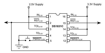
NOTE: The  $\overline{RST}_{2.5}$  volt output is connected to the IN<sub>3.3V</sub> via a 100k $\Omega$  resistor in the pushbutton input and therefore does not require a pull-up resistor (an addition pull up can be used to accelerate responses.) If an external pull-up is used in this example it must be connected to the 3.3V power supply.
