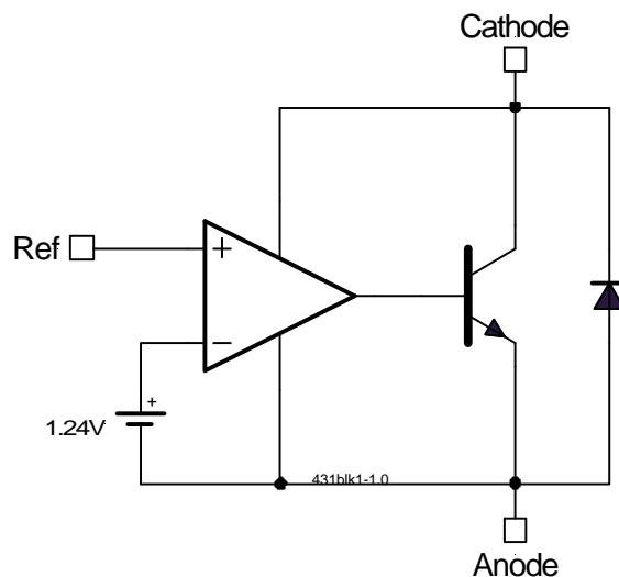
Figure 1 - Simplified block diagram of the IRU431L
