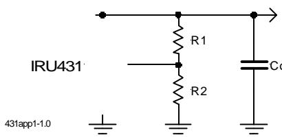
$$V_o = V_{ref} \times \left( 1 + \frac{R_1}{R_2} \right)$$
