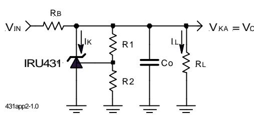
Figure 2 - Typical application of the IRU431L for programming the output voltage
