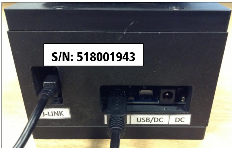
Figure 7: J-LINK cable connecting to programming jig
