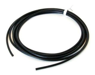
Coolflex45 cables get their name from the extremely low temperature rise under high current conditions. Testing under a continuous AC load of 45 Amps resulted in only a 30°F (17°C) temperature rise. Coolflex45 cables were also exposed to overcurrent loads of 70 Amps for fifteen seconds and resulted in only a 14°F (8°C) temperature rise. (Note, all testing was performed by an independent, certified laboratory)
