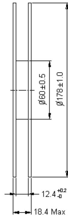
Note: 01. The tolerance unless mentioned is  $\pm 0.1 \text{mm}$
