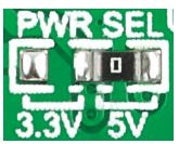
There is one zero-ohm SMD jumper **J1** used to select whether 3.3V or 5V power supply is used. Jumper **J1** is soldered in 3.3V position by default.
