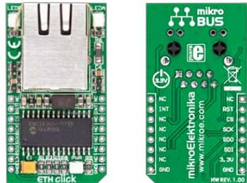
ETH Click is an accessory board in **mikroBus™** form factor. It features **ENC28J60**, a 28-pin, 10BASE-T stand alone Ethernet Controller with an on-board MAC & PHY, 8K Bytes of Buffer RAM and SPI serial interface. Chip supports programmable automatic retransmit on collision and automatic rejection of erroneous packets. Board contains standard RJ-45 connector, transmit, receive and power LEDs. On-board crystal oscillator ensures stable operation. Board is designed to use 3.3V power supply only.
