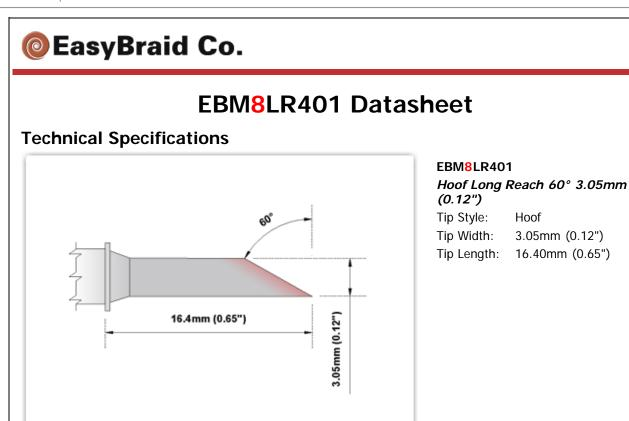
800 Type Cartridge<sup>1</sup>: 420°C - 475°C RoHS Compliant<sup>2</sup> / Lead Free: YES Equivalent to: SMTC-8170 For Use With: EB-9000S-1, EB-9000S-2, MX500 and MX5000
