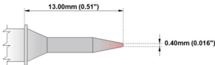
**ETM60CS150****Conical Sharp 0.4mm (0.016")**
