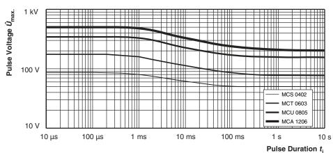
Maximum pulse voltage, single and continuous pulses; applicable if  $\hat{P} \leq \hat{P}_{\text{max.}}$ ; for permissible resistance change equivalent to 8000 h operation in standard operation mode
