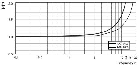
Relative impedance for 49.9  $\Omega$  chip resistor
