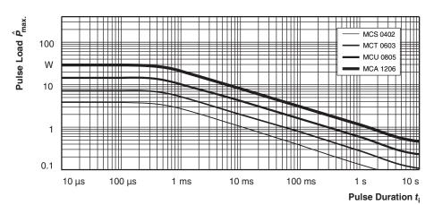
Maximum pulse load, single pulse; applicable if  $\bar{P} \to 0$  and n  $\leq 1000$  and  $\hat{U} \leq \hat{U}_{\text{max}}$ ; for permissible resistance change equivalent to 8000 h operation in standard operation mode
