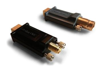
The dongles give users the flexibility to determine the best cable lengths for their applications. The transceiver contains an equalizer that is fully adaptive that adjusts to a variety of cable lengths as well as age and environmental conditions like temperature, without any need for programming. The dongles have a standard 1394b 9-pin connector on one end and a  $75\Omega$  BNC or  $50\Omega$  SMA connector on the opposite end.
