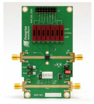
Figure 1. PE4312 Evaluation Board Assembly
