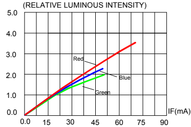
FIG.2 RELATIVE LUMINOUS INTENSITY VS. FORWARD CURRENT
